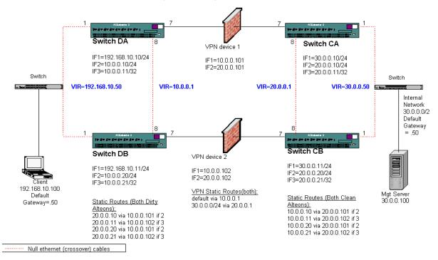
Figure 14-2 VPN Load-Balancing Configuration Example
